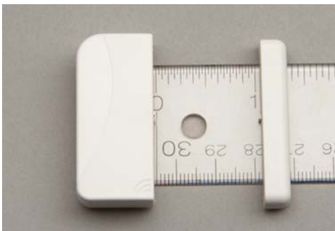
1-inch magnet gap; exceeding all sensors in the market
